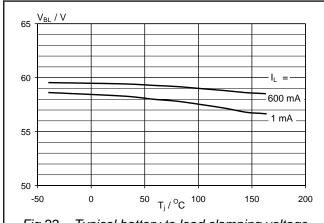
Fig.22. Typical battery to load clamping voltage.  $V_{BL} = f(T_j)$ ; parameter  $I_L$ ; condition  $I_G = 10 \text{mA}$
