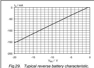
Fig.29. Typical reverse battery characteristic.  $I_{\rm G} = f(V_{\rm BG})$ ; conditions  $I_{\rm L} = 0$  A,  $T_{\rm j} = 25$  °C
